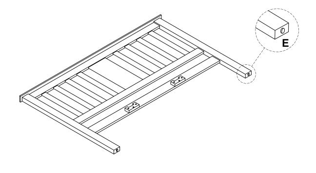
STEP 1: Attach 3 onto 1 and 2 using the bolts (B), tighten it up by using an allen key (D)
