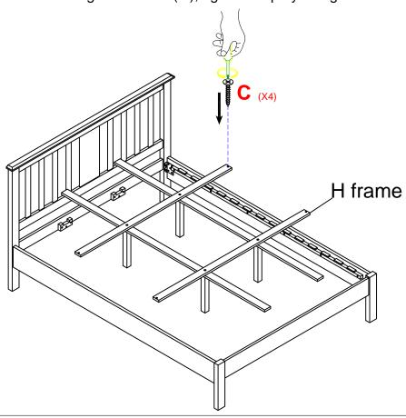
STEP 4: Attach 7 onto 3 using the screws (C), tighten it up by using an screwdriver.
